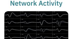
Raw voltage signals are processed in real-time to obtain extracellular field potentials from across the network, providing a valuable electrophysiological phenotype for applications in drug discovery, toxicological and safety screening, disease models, and stem cell characterization
