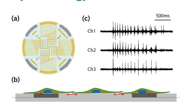
A planar grid of microelectrodes (a) interfaces with cultured neurons (b), modeling complex, human systems over an electrode array. Electrodes detect changes in raw voltage (c) through recording of extracellular field
